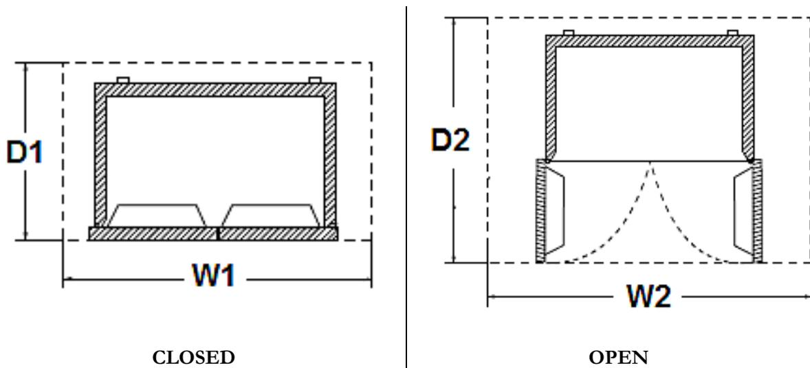
$$W 1 / W 2 = \text{Width} // D 1 / D 2 = \text{Depth}$$
