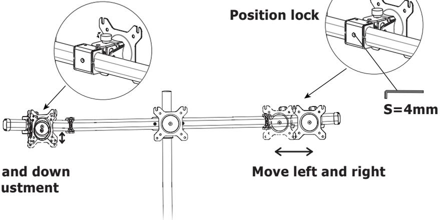
Move the display horizontally to a proper position and lock it using the wrench in the back of the plate.
