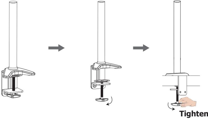
Loosen clamp screw until enough space is left for the edge of the desk.
