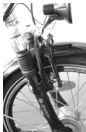
Suspension forks with elastomer/spring damping
