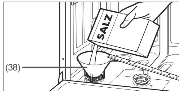
4. Place the supplied filling funnel (38) on the compartment opening.
