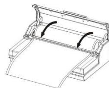
Put down the cutter rack and make sure it is on the right place of the bags, then slide the cutter from one end to the other end to cut the bag.
