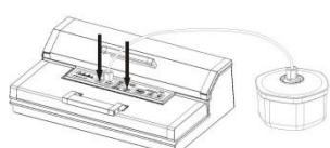
When the indicator light crush out, the marinate process is completed. Pull off the hose accessory from canister port and canister cover.
