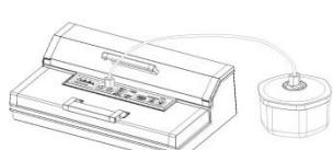
Insert one end of the hose into the air intake and another end of the hose into the center hole of the canister cover.
