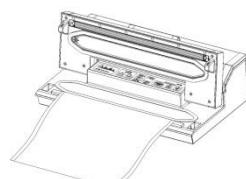
Put one end of the bag on top of the sealing profile, but not enter the vacuum chamber.
