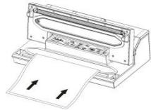
Place the open end of the bag within the vacuum chamber area. Make sure the air intake is not covered by the bag.
