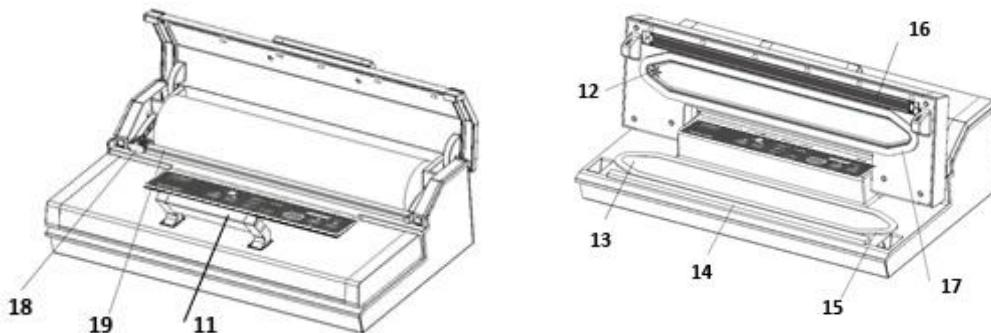
**11. Front handle:** Press down to lock the cover. And lift to open the cover.
