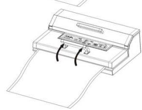
Lift the front handle to open the cover and take the bag out of the machine. The bag is then done and is ready for vacuum sealing .
