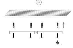
Align, mark & drill hole, apply plastic anchors & tie up the screws
