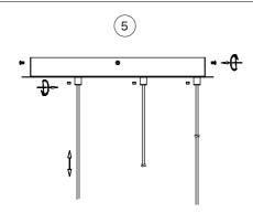
Apply side screws & adjust the cable
