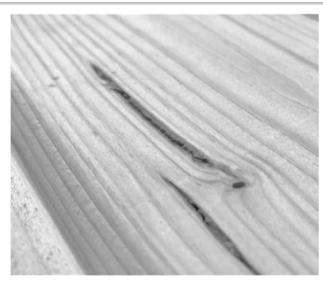
Examples of the allowed defects of filler strips :
