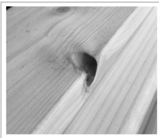
Examples of the allowed defects of filler strips :
